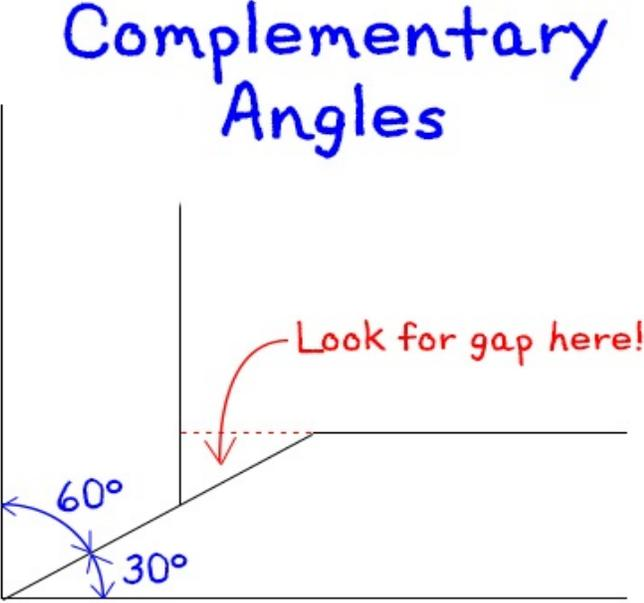
The reason you flip one piece of moulding is so each corner adjustment is considered separately. When you flip, you are actually adding Corner A to Corner A, which means the measured error will be twice as much as the actual error, making it easier to measure.
