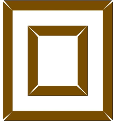
2. When you are comparing the lengths of opposite pieces, and you have them side by side with the miters face up and their back sides touching, you may notice by running your finger over the miter that they are the same length on one end of the miter but not the other, or that one piece of moulding is higher at one end of the miter and the other piece is higher at the other end.
